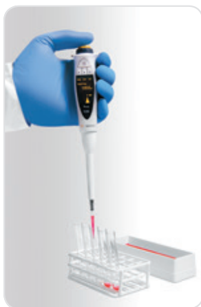
Hold the pipette in a vertical position during aspiration.
