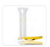
This filter holder is available in two versions differing from each other only in the type of the filter support. The filter with glass frit ensures uniform distribution of retained particles and is therefore recommended when the residue on the filter surface is of interest. Because it is easy to clean, the device with the PTFE-coated screen support is preferable when the filtrate is required, or when liquids difficult to remove from glass frits must be examined. The PTFE ring, which holds the
