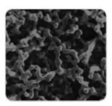
Polyamide membrane filters are hydrophilic and chemically resistant to alkaline solutions and organic solvents. They are therefore recommended for the particle removal from aqueous solutions and solvents for analytical determination such as HPLC, for the sterile filtration of these liquids as well as for applications where a membrane with a relatively high nonspecific adsorption is suitable.
