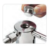
A practical filter holder for many laboratory filtrations. It can be attached to a tripod with the help of a steel rod which can be screwed in. The hose nipple is screwed into the side of the top part, leaving room for a large filling opening. This makes pouring in the sample easier, and the sample can be refilled without removing the tube connection to the pressure source. Leak-proof sealing is achieved by
