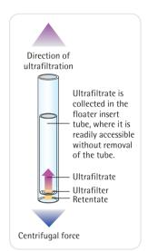
Centrisart® I\* is a ready-to-use unit for small-volume, centrifugal ultrafiltration to separate proteins from low molecular weight substances in biological samples.
