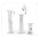
Vivapure® Mini-400 | 500 μl Binding capacities: 1 mg to 4 mg
