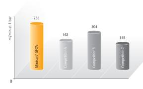
$0.45~\mu m$  SFCA membrane compared with CA (Cellulose Acetate) or similar hydrophilic membranes of the same pore size
