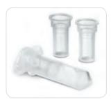
Vivaclear centrifugal filters are disposable microfiltration devices for the fast and reliable clarification filtration of biological samples in the range 100  $\mu l$  to 500  $\mu l$ . They can be used in fixed-angle rotors accepting 2.2 ml centrifuge tubes.
