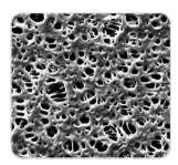
Polyethersulfone (PES) membrane filters are hydrophilic, have high flow rates thanks to their symmetric structure, have a low non-specific protein adsorption and are chemically resistant over a pH range of
