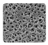
The very low adsorption membranes are hydrophilic, solvent-resistant (pH 3-12) and therefore suited for the particle removal from solvents. The membrane is asymmetric and reinforced with nonwoven cellulose. They are available in two pore sizes: 0.45  $\mu m$  and 0.2  $\mu m$ .
