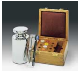
Permeability indicator for testing the magnetic properties of weights
